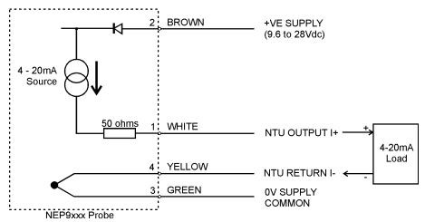
For very long cable runs (>200m), it may be advisable to connect the the NTU Return conductor to the Supply Common conductor at the end of the cable to reduce the voltage drop along the run.
