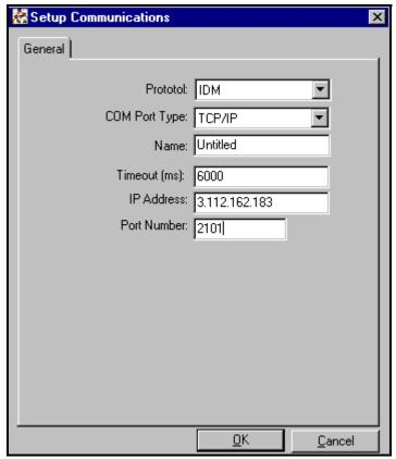
Figure C-3: Setup Communications for TCP/IP
