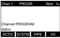
Press the  $[\leftarrow]$  and  $[\rightarrow]$  keys and a function key [F1]-[F4] to select the desired submenu. From this screen, press [EXIT] to return to the initial *User Program* screen shown on page 1-8.
