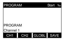
Press the  $[\leftarrow]$  and  $[\rightarrow]$  keys and one of the function keys [F1]-[F4] to select the desired submenu. From this screen, press [EXIT] to return to measurement mode.
