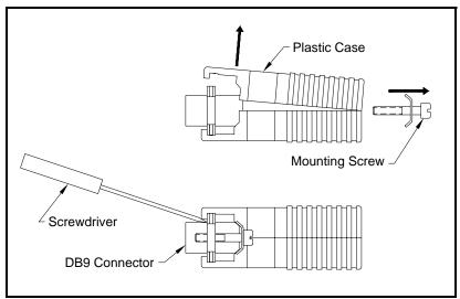
Figure 6-2: Opening the Converter Case
