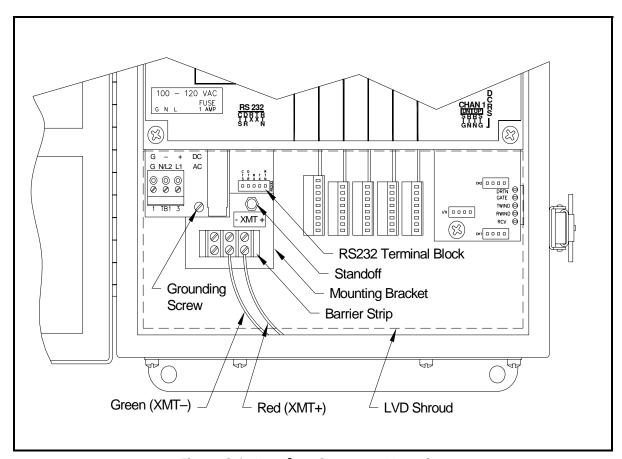
Figure 6-1: Interface Converter Mounting
