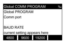
To change the baud rate, press the  $[\rightarrow]$  key until the desired baud rate appears on the option bar, and then press the appropriate [Fx] function key.
