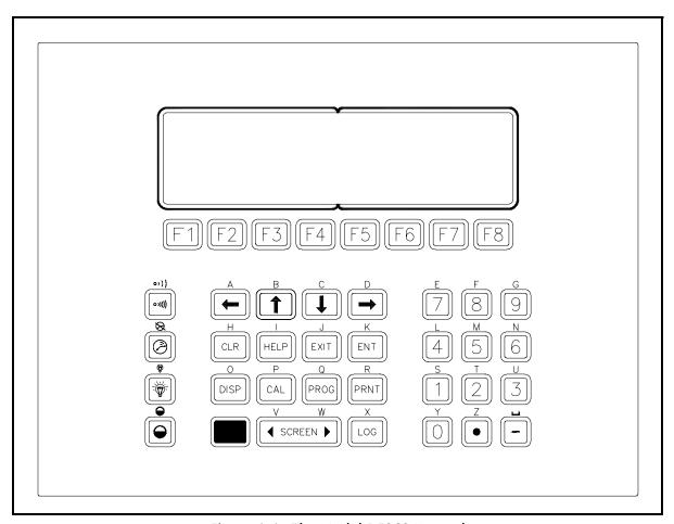
Figure 1-1: The Model DF868 Keypad
