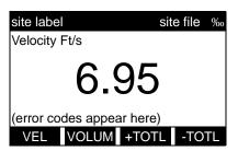
The default power up screen is already in BIG mode. If a different display mode is active, access the *Display Menu* by pressing the [DISP] key.
