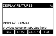
Press [F1] to select the BIG option. The measurement mode screen reappears with the display in the BIG format.
