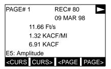
Use the  $[\leftarrow]$ ,  $[\rightarrow]$  and [F1]-[F4] keys to view additional records or to exit the log display. The options are listed in Table 2-3 below.
