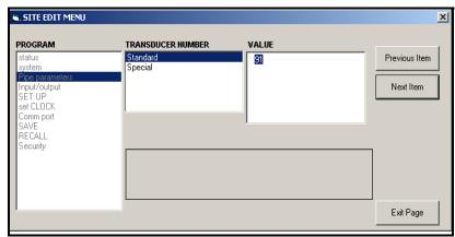
Figure C-21: Pipe Parameters Option in Site Edit Menu
