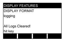
There are no log files currently stored in memory. Either all of the log files have been cleared or no log files have yet been created. Press any key to return to measurement mode.
