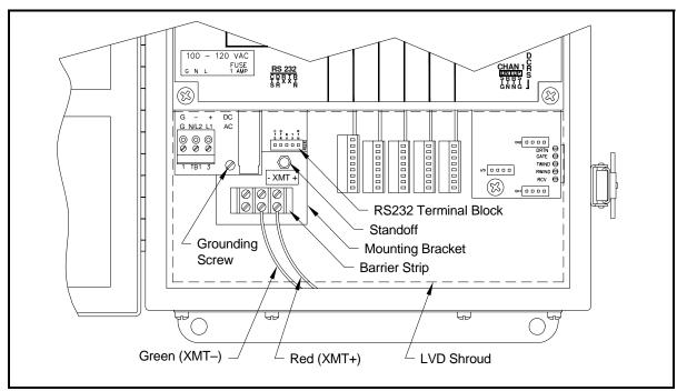
Figure 6-1: Interface Converter Mounting
