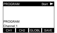
Press the  $[\leftarrow]$  and  $[\rightarrow]$  keys and one of the function keys [F1]-[F4] to select the desired submenu. From this screen, press [EXIT] to return to measurement mode.
