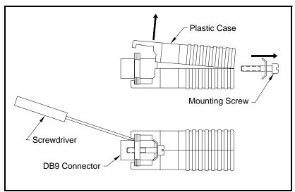
Figure 6-2: Opening the Converter Case
