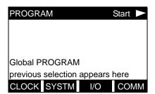
Press the  $[\leftarrow]$  and  $[\rightarrow]$  keys and a function key [F1]-[F4] to select the desired submenu. From this screen, press [EXIT] to return to the initial *User Program* screen shown on page 1-8.
