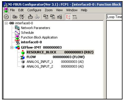
Figure D-1: Configuration Utility Setup Example
