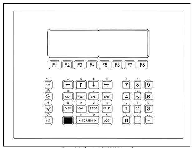
Figure 1-1: The Model GS868 Keypad
