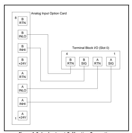
Figure 1-3: Analog Input Calibration Connections
