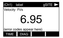
Press the  $[\leftarrow]$  or  $[\rightarrow]$  keys until DIAG appears on the option bar. Press the appropriate [Fx] key to select this option.
