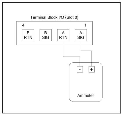
Figure 1-1: Ammeter Connection for Slot 0 (Output A)
