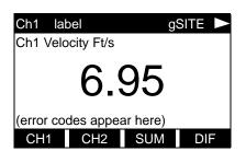
Press the  $[\leftarrow]$  or  $[\rightarrow]$  keys until the desired channel option appears on the option bar. Press the appropriate [Fx] key to select this option.
