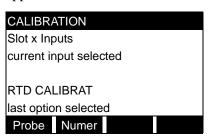
Press [F1] to select the Probe method of calibration, or [F2] to select the numeric method.
