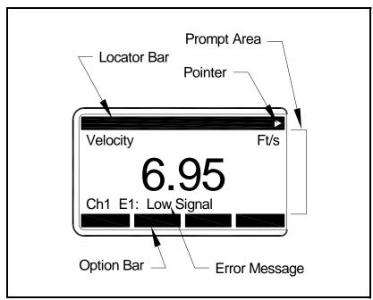
Figure 2-1: A Typical Display Screen
