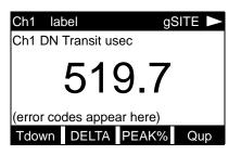
Press the  $[\leftarrow]$  and  $[\rightarrow]$  keys and the appropriate [Fx] key to display a different diagnostic parameter or to EXIT the *Diagnostics Menu*.
