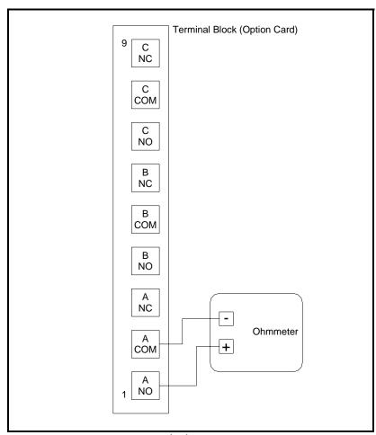
Figure 1-4: Typical Ohmmeter Connections
