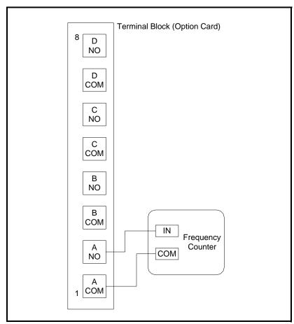
Figure 1-5: Frequency Counter Connections
