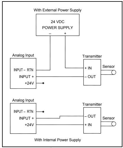
Figure 5: Analog Input Wiring Diagram
