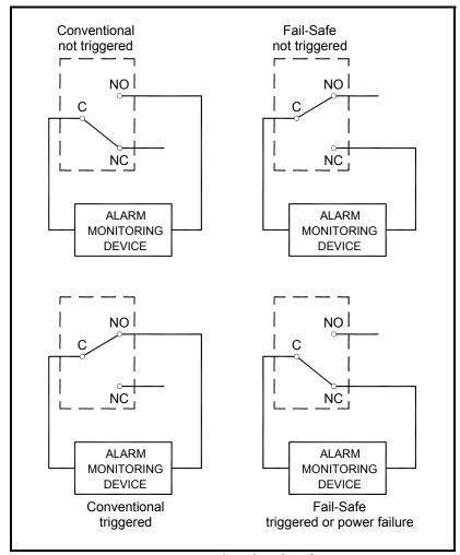
Figure 4: Conventional and Fail-Safe Operation
