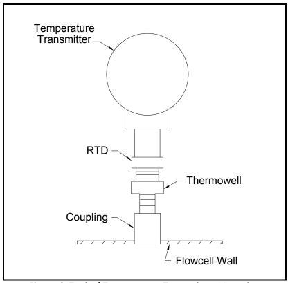
**Figure 2: Typical Temperature Transmitter Mounting**
