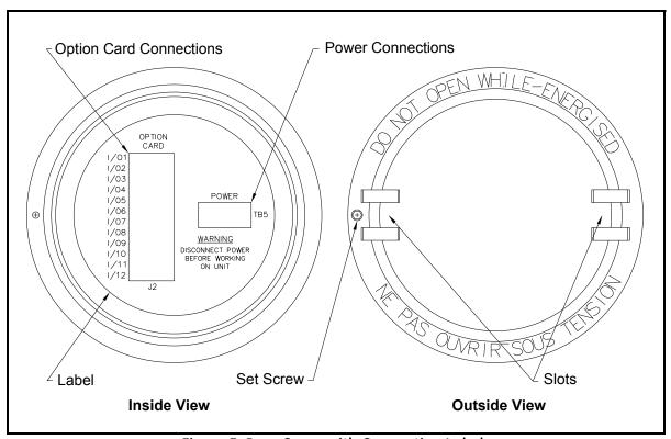
Figure 3: Rear Cover with Connection Labels
