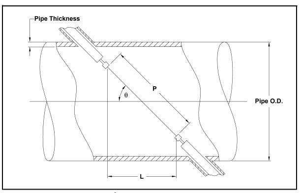
Figure 22: 180° Transducer Installations - Top View
