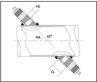
Figure 23: Determining the Pipe Coupling Length
