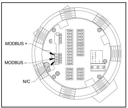
Figure 7: The RS485 MODBUS Terminal Block Connector
