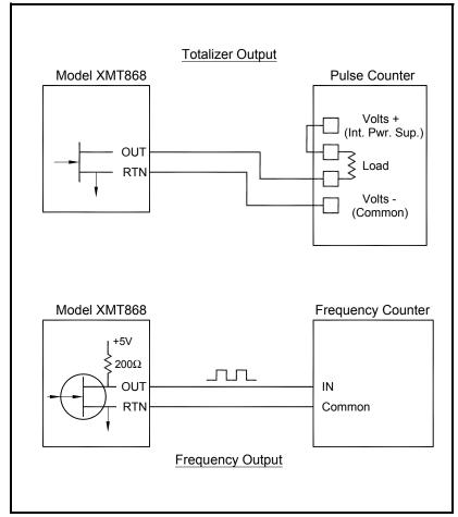
Figure 6: Totalizer and Frequency Output Wiring
