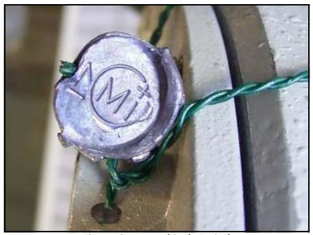
Figure 42: NMI Lead Seal - Typical
