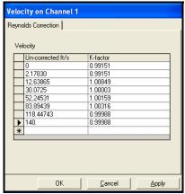
Figure 36: Velocity/K-Factor Table
