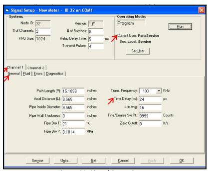
Figure 20: Signal Setup Screen
