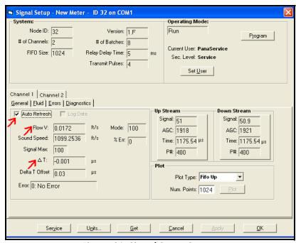
Figure 21: Signal Setup Screen
