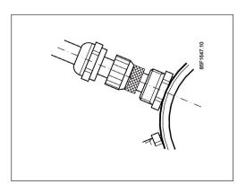
For connection of the 4 cables, just carefully press the cable into the cable glands until the "snap function" **fixes** the cable inside the connection module. Make sure the cable is mounted correctly by smoothly pulling the cable.
