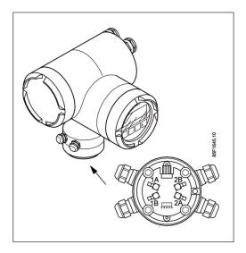
When opening the lid you will have direct access to checking the correct transducer cable connections.
