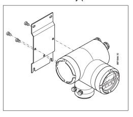
The mounting bracket is suitable for wall assembly only.
