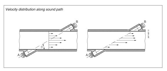
A sound wave travelling in the same direction as the liquid flow arrives at point B from point A in a shorter time than the sound wave travelling against the flow direction (from point B to A). The difference in sound transit time indicates the flow velocity in the pipe.
