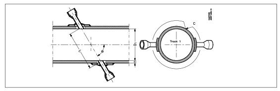
This parameter is the distance between the ultrasonic transducers, as illustrated in the picture. The value is necessary in order to calculate the ultrasonic velocity from the time of flight and the distance between the transducers.
