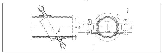
For SONOKIT: Data to be entered from "SENSOR GEOMETRY MEASURING REPORT" If it is a 2-track SONOKIT, use same procedure for track 2.
