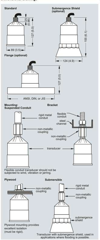
XRS-5 ultrasonic transducer, dimensions, in mm (inch)
