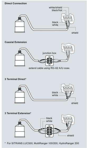
XRS-5 ultrasonic transducer connections
