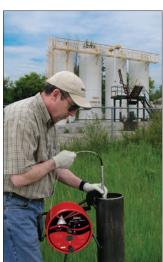
If the liquid is a non-conductive oil/product the signals are steady. If the liquid is water (conductive liquid greater than 20  $\mu S/cm),$  the conductivity of the water completes a conductivity circuit. This overrides the infra-red circuit, and the tone and light are intermittent.
