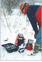
750ft. (230m) Waterloo System installation for a deep tunnel assessment study. Three zones monitored with dedicated Double-Value Pumps and pressure transducers. Picture shows technician obtaining pressure measurements and groundwater samples with portable readout and pump control unit.
