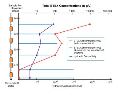
Underground oil pipeline leak assessment. Three 150 ft. (45m) installations. Two point rising head permeability tests were conducted in each interval of the Multilevel System. (See diagram showing contaminant distribution at left.)
