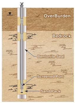
Direct Placement: Sand and Bentonite with Screened Ports
