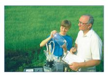
A large Midwestern USA research project studying agricultural effects on water quality. 22 Waterloo System installations with 3-4 zones each were installed to depths of 24-60 ft. (7.3-18.3 m) in overburden. Dedicated Double Valve Pumps and Peristaltic Pumps were used.
