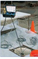
An EPA regulated site in Northeast, USA. This multilevel array allowed a sampling team to purge and sample from 40 monitoring zones across 10 borehole locations in just 4 days. These Waterloo Systems were installed in overburden using preinstalled casing.
