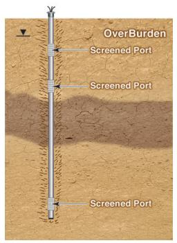
Direct Burial: Formation Collapse with Screened Ports
