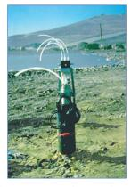
Landfill site over fractured granite, monitored with five Waterloo Systems. Each System comprised of dedicated Double Valve Pumps and Pressure Transducers in 4-6 intervals to depths of 275 feet (84m). The Multi-Purge Manifold allowed the monitoring of 21 zones to be completed in less than 2 days.
