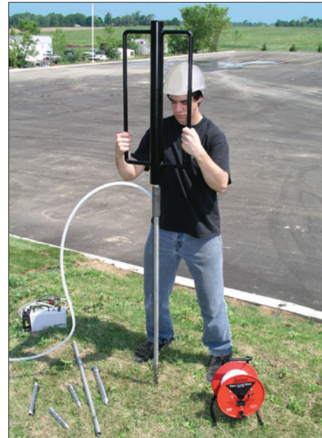
Installing Piezometers with a Manual Slide Hammer
