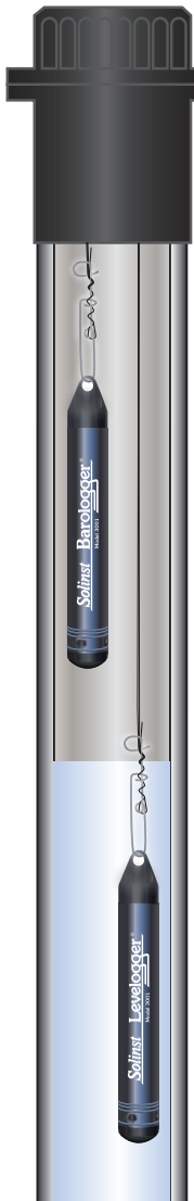
Figure 10-12 Levellogger and Barologger in Well
