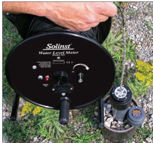
Measure Water Levels within the narrow channels of a Solinst CMT® System.
