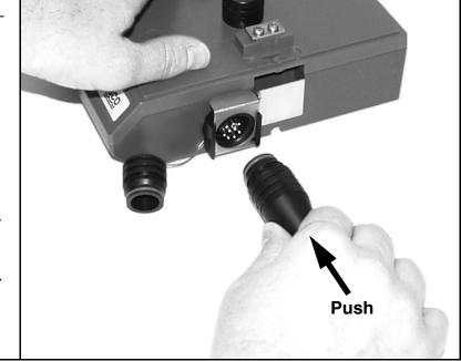
Figure 1-10 Flow Module - Connecting the Probe
