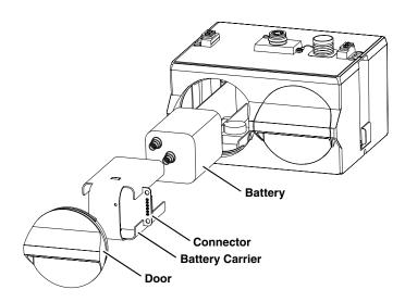
Figure 3-1 Installing a Battery
