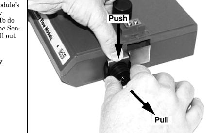
Figure 1-9 Flow Module - Preparing the Probe Connectors
