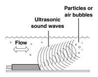
The 2150 measures liquid level and average stream velocity, and calculates the flow rate and total flow. The liquid level and velocity measurements are read from an attached AV Sensor that is placed in the flow stream. Flow rate calculations are performed internally using the measured parameters from the AV Sensor. Additionally, the AV Module can measure its input voltage – a service feature.
