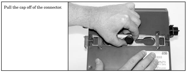
Figure 1-18 Flow Module - Uncapping the Connector
