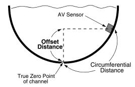
Figure 4-3 Zero Level Offset Measurement
