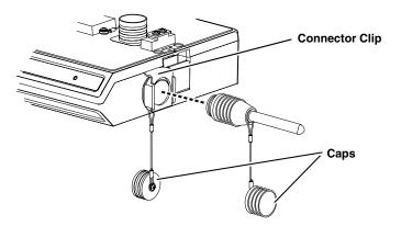
Figure 3-3 Connecting the AV Sensor
