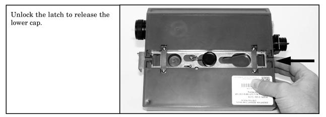
Figure 1-17 Flow Module - Unlocking the Latch
