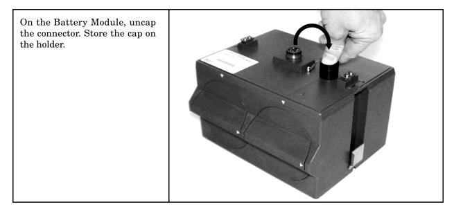
Figure 1-20 Battery Module - Uncapping the Connector
