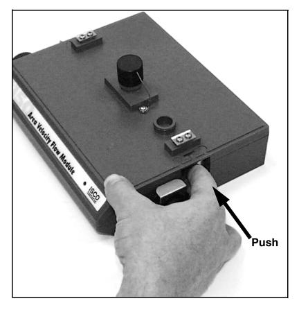
Locate the latch release on the right side of the module. Push in to slide the latch toward the left of the module.
