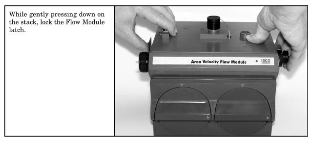
Figure 1-23 Aligning the Modules: Push Down and Lock the Latch
