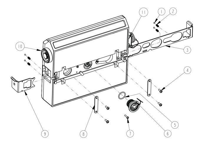
DRAWING NO. 602003112 D sheet 1 of 5 REPLACEMENT PARTS LIST, 2150 AREA VELOCITY MODULE
