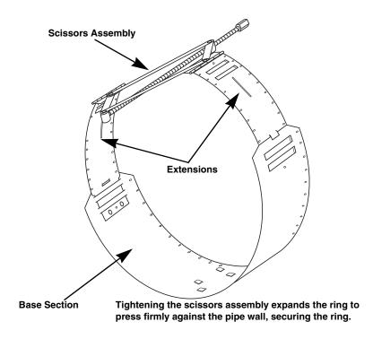
Figure 3-6 Scissors Ring adjustment
