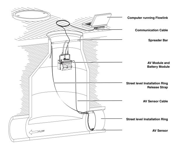
Figure 3-4 Typical Round-pipe Installation
