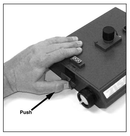
Locate the latch extending from the left side of the module. Push in to slide the latch toward the right of the module.
