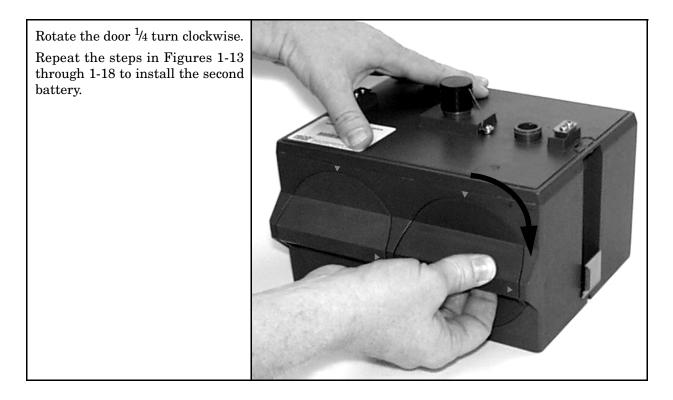
Figure 1-16 Battery Module - Closing the Door
