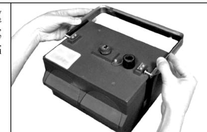
Figure 1-21 Battery Module - Inserting the Handle
