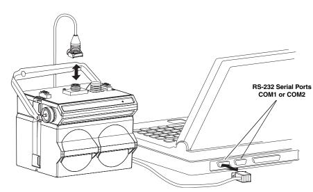
Figure 4-1 Flowlink connections
