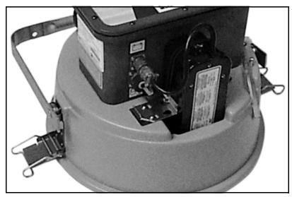
Figure 2-4 Nickel-Cadmium Battery and Power Pack Position
