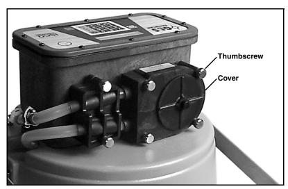
Figure 2-1 Pump housing cover and thumbscrews
