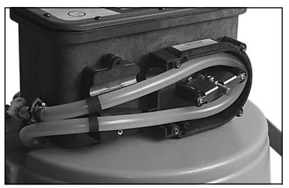
Figure 5-1 Liquid detector and pump housing covers removed
