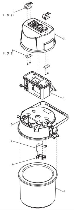
Flat Washer, #6, Lock Washer, #6, Screw, 8-32 x 3/4 (4) For mounting controller to center section.
